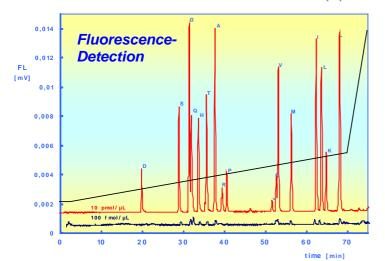
Stationary phase: GROM Sapphire 110 C18, 3  $\mu m$  Column: (a, b) 150 mm x 2 mm, (c) 150 mm x 0.3 mm
